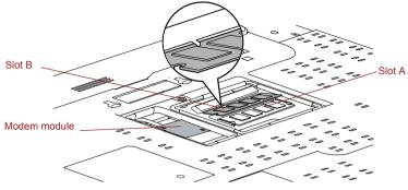
Figure 3-7 Seating the memory module
